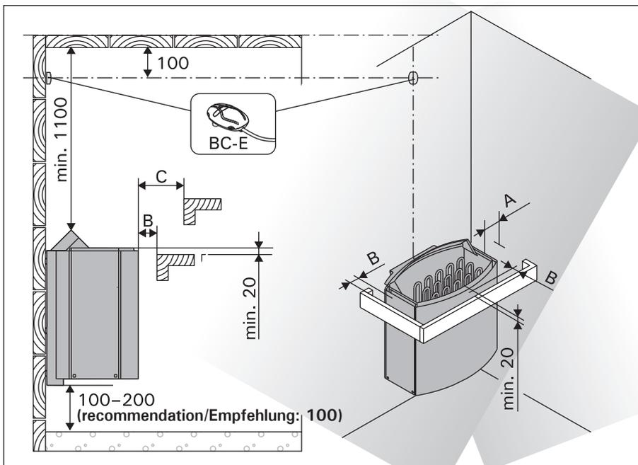
The heater can be mounted in a recess with a minimum height of 1900 millimetres.
