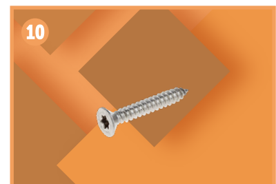
Stacks [1SP11-01-044] Screw 6.3x45 ISO 14586, drill 5 mm, TX30 (number according to number of stacks)
